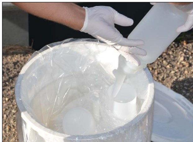
FIGURE 1 – POURING A FIELD BLANK SAMPLE
