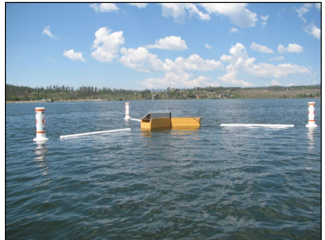
Figure 2. Real-time water quality monitoring buoy in Shadow Mountain Reservoir.
