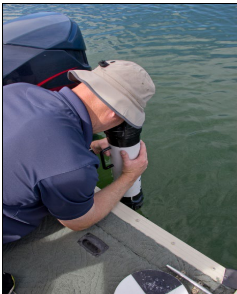
Figure 3 - Measuring Secchi depth with a view scope
