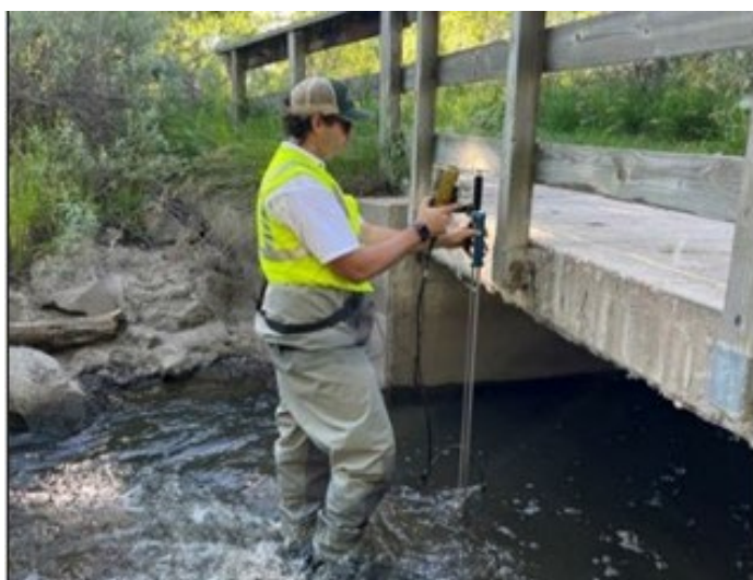
Figure 3. Manual flow measurement in the Poudre River
