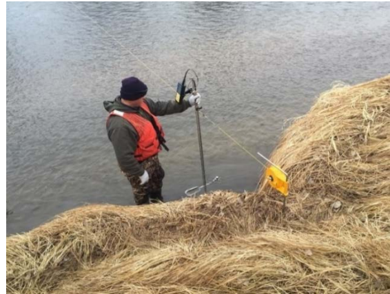
Discharge Measurement on the Poudre River
