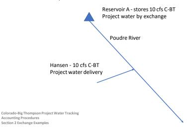
Example 3 Description – Diversion of C-BT Project water at Ditch 1 by exchange from Reservoir A (Reservoir A is a Non-C-BT Project storage structure in this example)
