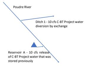
Colorado-Big Thompson Project Water Tracking Accounting Procedures Section 2 Exchange Examples Example 4 Description – Diversion of C-BT Project water at Reservoir B by exchange from Reservoir A (This can occur two ways, first by physically storing 10 cfs in Reservoir B and second by relocating C-BT Project Water if Reservoir B already has other water stored in it. Reservoir A and B are Non-C-BT Project storage structures in this example)
