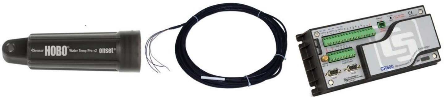
Figure 3 - Temperature monitoring equipment.
