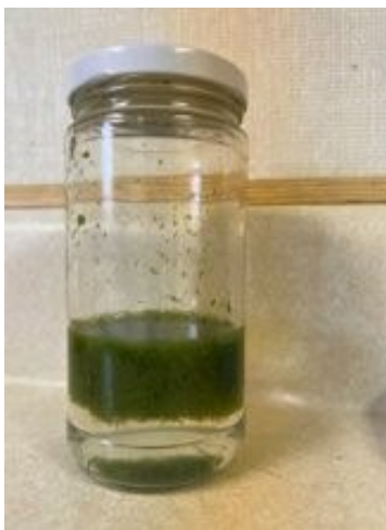
Figure 7. Image of a jar that indicates likely presence of cyanobacteria.
